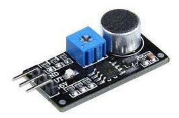
The sound sensor module provides an easy way to detect sound and is generally used for detecting sound intensity. This module can be used for security, switch, and monitoring applications. Its accuracy can be easily adjusted for the convenience of usage.
