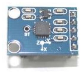
**GY-61 DXL335 3-Axis Accelerometer Module** is a three axis accelerometer sensor module based on ADXL335 integrated circuit. The ADXL335 is a triple axis accelerometer with extremely low noise and power consumption. The sensor has a full sensing range of +/-3g. It can measure the static acceleration of gravity in tilt-sensing applications, as well as dynamic acceleration resulting from motion, shock, or vibration.
