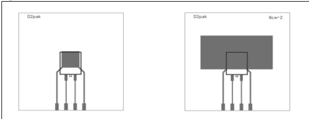
Figure 39. D 2 PAK PC board (1)
