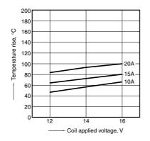
1-(3). Coil temperature rise (at room temperature)
