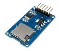
The module (Micro-SD Card Adapter) is a Micro SD card reader module, and the SPI interface via the file system driver, microcontroller system to complete the Micro-SD card read and write files. Arduino users can directly use the Arduino IDE comes with an SD card to complete the library card initialization and read-write.
